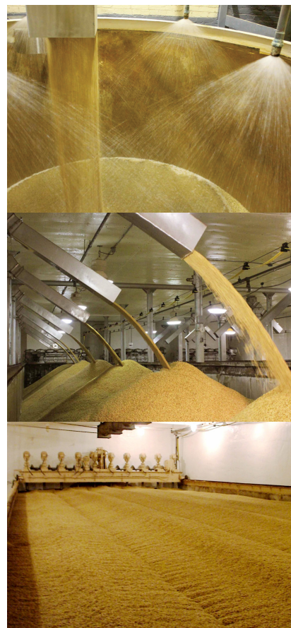
Top to bottom: Barley is sprayed and soaked in water to bring up the moisture content; transferring the sprouting malt out of the steeping tanks; a mechanical turning device rests at the far end of the malting floor. Photos courtesy of Briess Industries, Inc.
