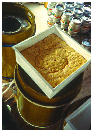
Many traditional British fermenters incorporate special devices to force yeast up into a space from which it can be collected and re-pitched, assuring vigorous top-fermenting behavior. This setup was in a small brewery in Kent.
